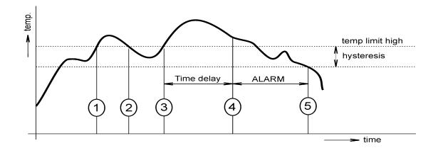
An alarm report is always sent right after an alarm appears. The device memorizes sent alarm reports of current alarms while the power is connected. In case of power disconnection or a reset of the device (e.g. by modification of configuration) a new alarm evaluation is performed and new alarm reports are sent again, if any.
