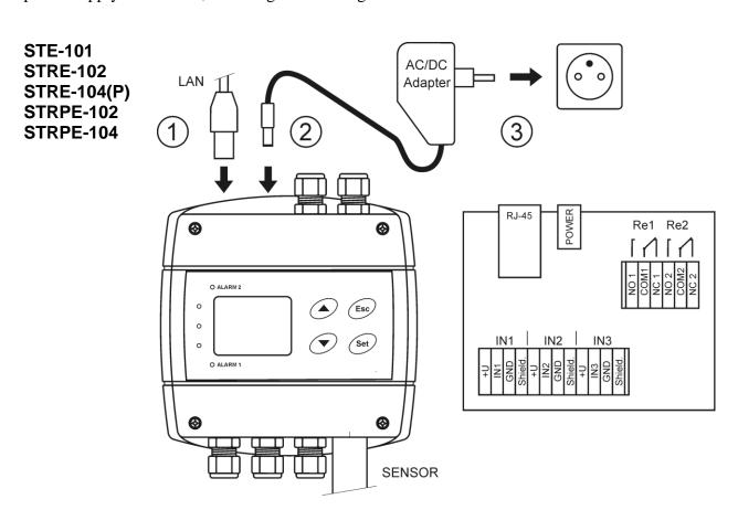
Binary inputs are not galvanic isolated, connection terminals +U are internally connected to the device power supply (ie. the +U terminals provide the same voltage level as power supply).
